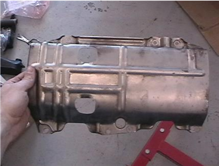
Next the windage tray needs to be installed onto the engine. Here is the windage tray, and windage tray installed:
