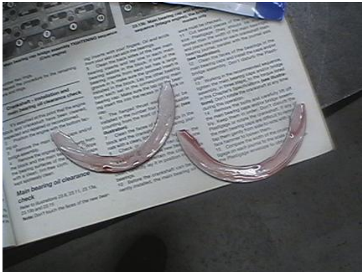
Pictured is the thrust washers with the lubricant helping attaching them to the metal surface. Note the thrust washers groove facing outward:
