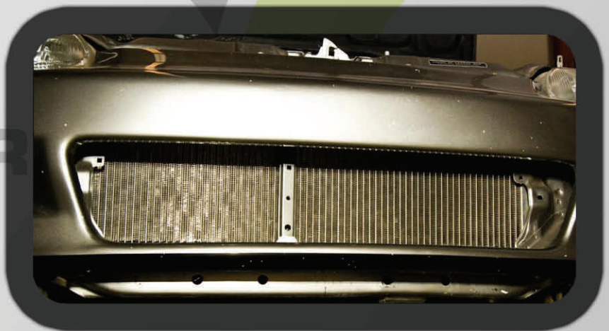
(right) Hybrid Racing Full-Size K-Swap Radiator for EG Civic. As viewed from front of car.
