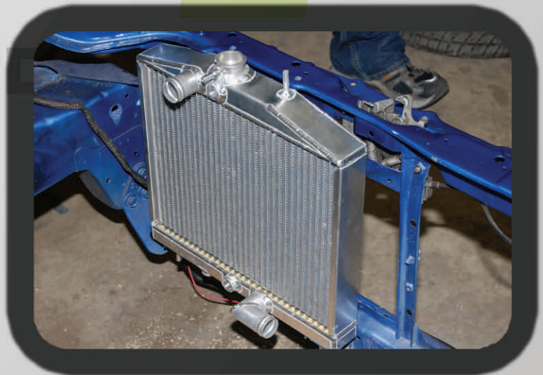
(right) Hybrid Racing Half Size Radiator installed in EG chassis
